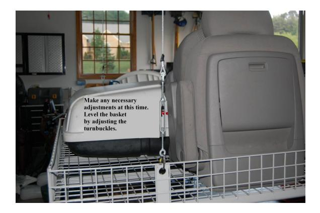
Now lower the basket by turning the master switch to the down position and press and hold the down button until the basket either stops or hits the ground.
